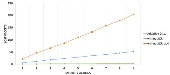
Figure 2. Results comparing accumulative lost packets when applying normal vs. adaptive data dissemination
